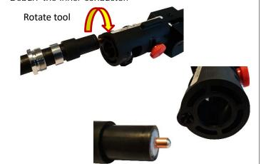
(5) Dismantle the cable 20 mm. Preset on tool.
