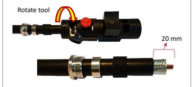
6 Insert braid fixator (connector part) between foil and braid until stop. Do not force it underneath the outer sheath. No need to heat up the cable!
